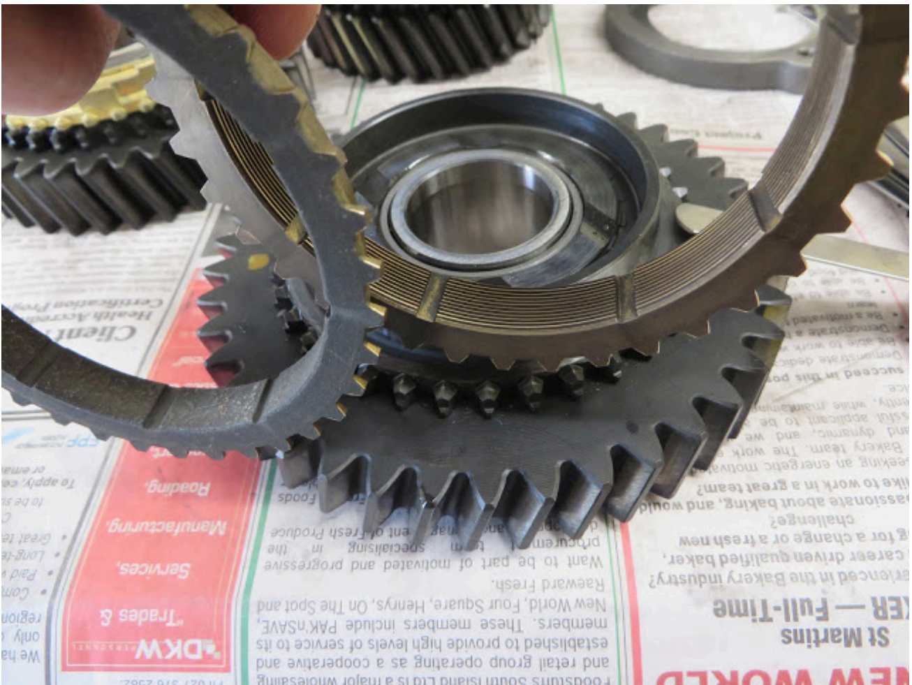
Next up is the synchro rings for a measure up, reverse on the left fwd synchro rings on the right.
