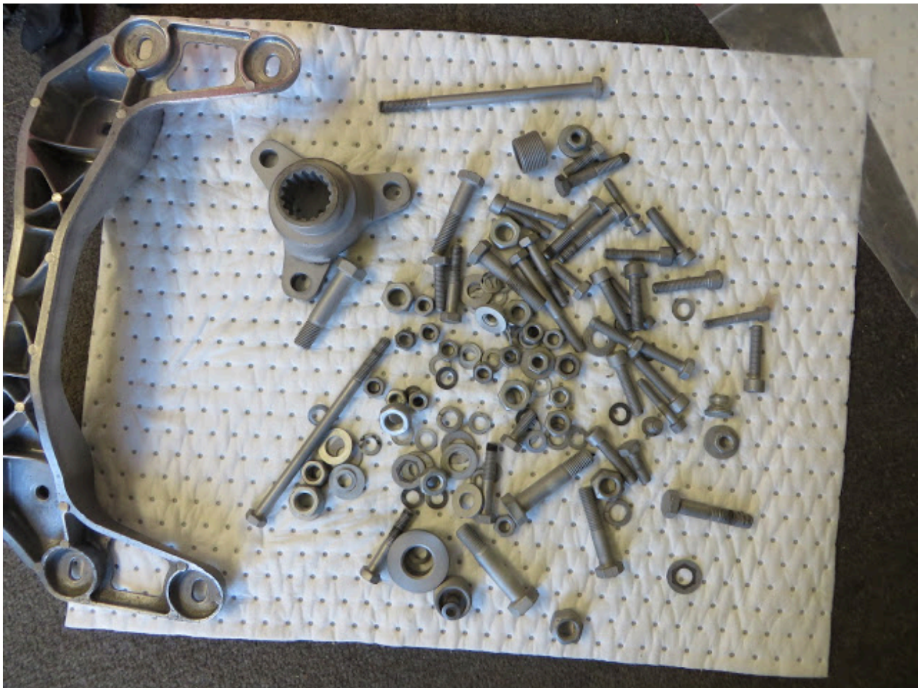
I bead blasted the hardware parts (cross member not included) and then they were gold Zinc coated, shown in one of the above photos.
