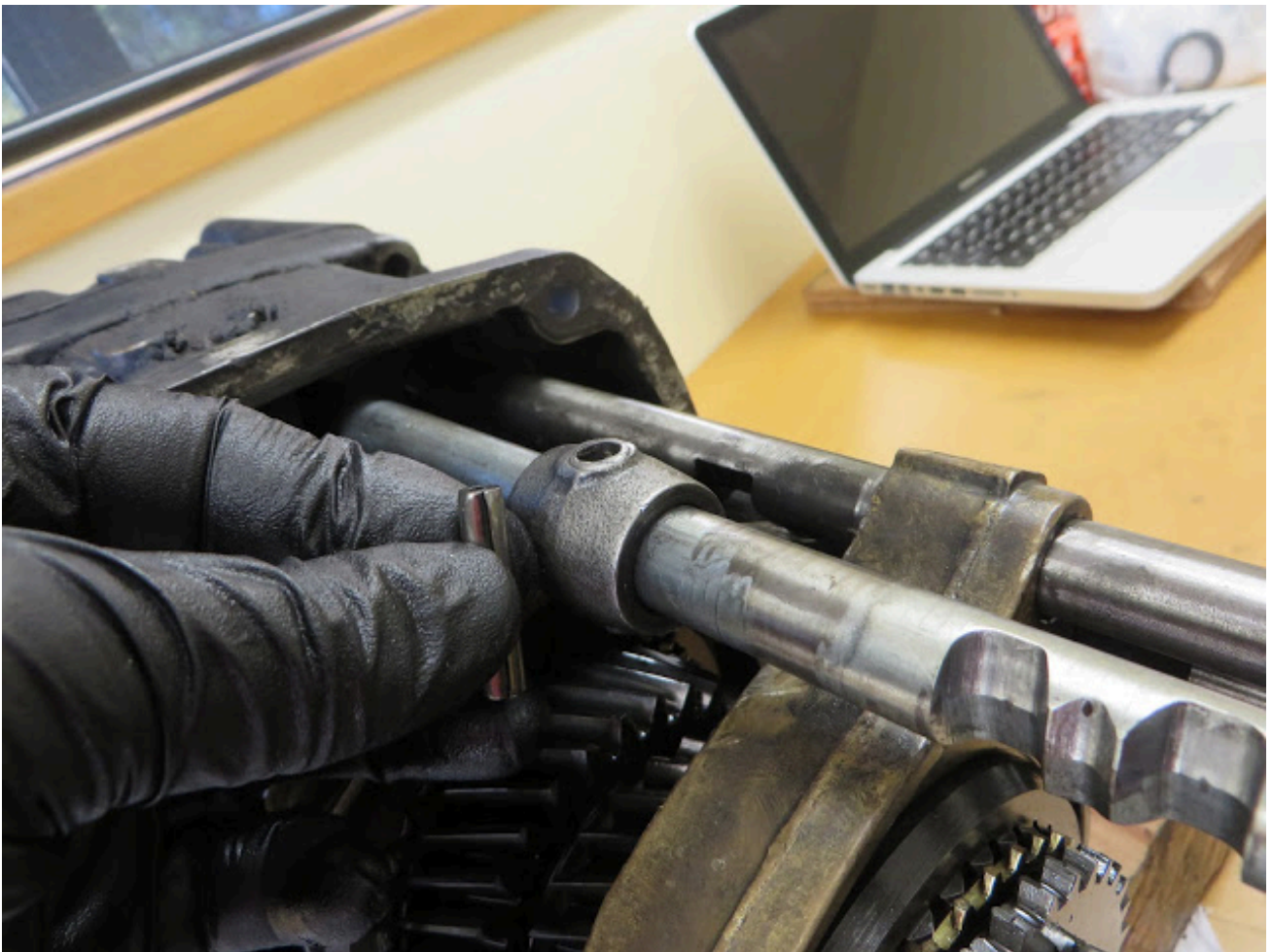
Had to remove the roll pins, 2nd 3rd hub roll pin is tricky to remove it basically hammers down the gap between the gear teeth.
